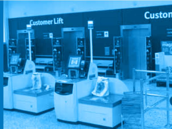
The system requires the labels to be attached to product which are then “blown” when passed through the checkout using deactivation from underneath the till. If the product is taken out of store without passing through the checkout then the antennae will detect the EAS tag and set off an alarm. This will also trigger linked CCTV cameras to hone in on the individual in question, and automatically bookmark the relevant CCTV footage.
